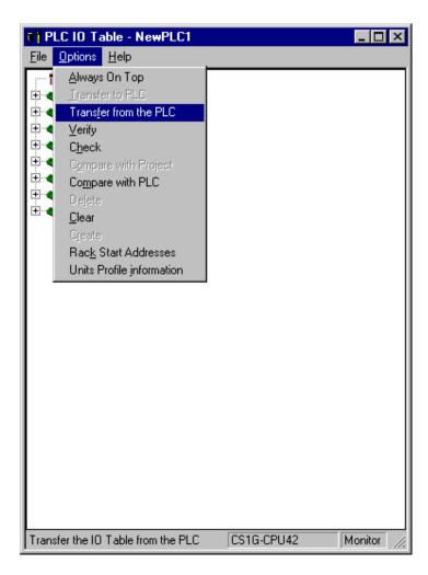
When IO Table is received, display the slot list under Main Rack (press "+" button in the "PLC IO Table - NewPLC1" dialog box). Select "Ethernet Unit(ET)(0)" and press the mouse right button. The Ethernet Unit menu appears:
